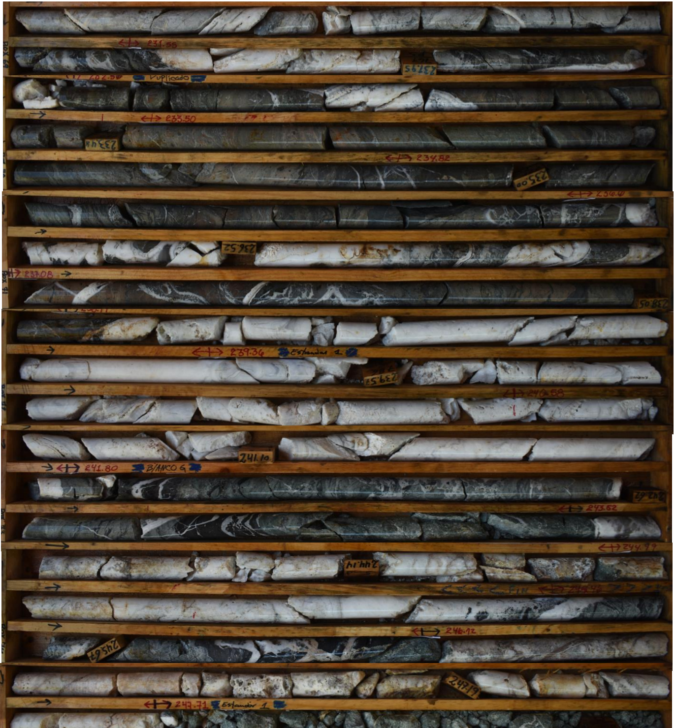
Zone of quartz-calcite veining and stockworks hosted in Mcv tuffaceous volcanics (Veins VS_01 & VS_21)
